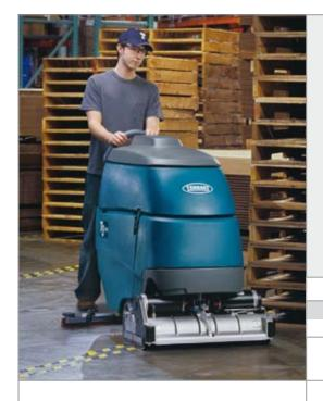
High productivity with gel batteries. Achieve up to 5 hours of run-time with environmentally-preferable sealed batteries.
